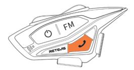
If you do not need the auto-answer function, When not connected to Bluetooth, you can double-click press the [on/off] key to cancel or open the auto-answer function (the initial state of the default auto-answer); (Indicator status: flashing blue light two times to open auto-answer, and flashing red light two times to close auto-answer.)
