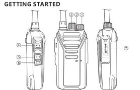
① Power/Volume Knob otating to adjust the volume. To turn it off, rotate the knob end anticlockwise. background noise while adjusting volume. ② LED Indicator When transmitting, LED indicator turns green, and when 3.Channel Select
